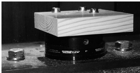
Figure 1: The load-cell, marked ATI, and work-piece setup in the milling machine. Photo by Jan Palmqvist.
