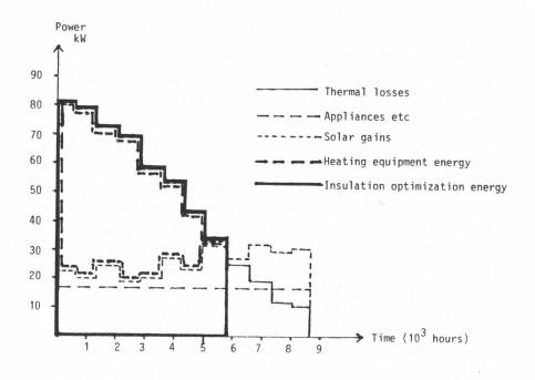
Figure 1. Duration curve for residential heating.
